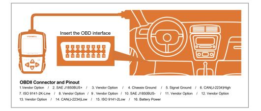
In the main menu, ENTER OBDII/EOBD. The code reader will start scanning. Wait several seconds, then choose "yes/no" with the right arrow key, and enter the Diagnostic Menu.
